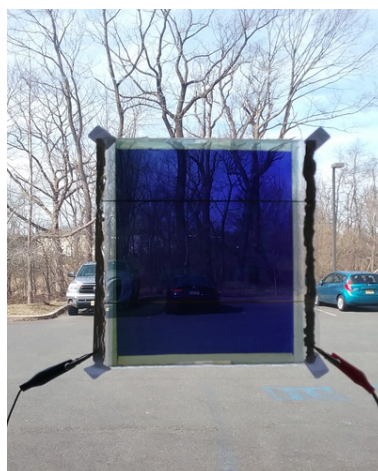
Electrochromic Panel made by Screen Printing mounted in window, DARK state
