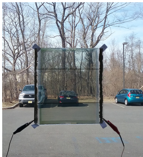
Electrochromic Panel made by Screen Printing mounted in window, LIGHT state
