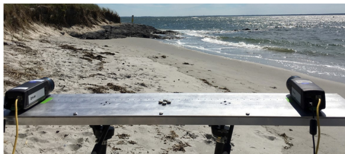
This photo shows two cameras equipped with ThermalTracker software, which is designed to capture the flight patterns of birds and bats and provide more accurate data about their behavior around offshore wind turbines. Photo courtesy of PNNL
