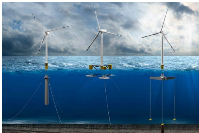
Offshore wind floating substructure designs: spar buoy (left), semisubmersible (middle), and tension-leg platform (right). Image by Josh Bauer, NREL 49054
