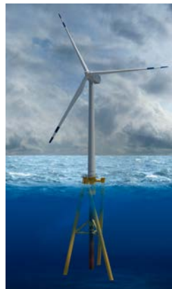
Offshore wind turbine with twisted jacket foundation. Illustration by Josh Bauer, NREL 500052
