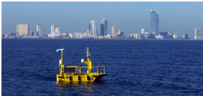
A lidar buoy deployed off the coast of New Jersey has provided observational data that, in conjunction with data from another buoy, will help inform wind production capability for offshore locations. Photo courtesy of PNNL
