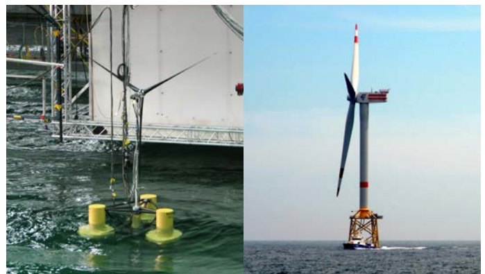
OC5 focused on validation by comparing simulated results to actual measurements. Its three phases used test data from a cylinder in a tank, a floating semisubmersible prototype turbine and substructure in a tank (left), and the open-ocean testing of a jacket foundation (right). The IEA Wind Technology Collaboration Programme's Executive Committee recently awarded a 4-year extension of IEA Wind Task 30, creating OC6. Photo credits: (Left) DeepCwind Research Program, NREL 19576; (Right) Gary Norton, NREL 27360
