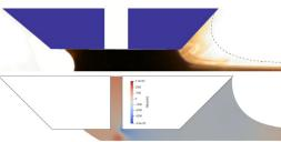
Validation of single-layer slot coating deposition (flow visualization in literature)
