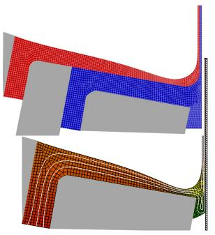
Two-layer and single-layer predicted pattern of flow and free surface shape
