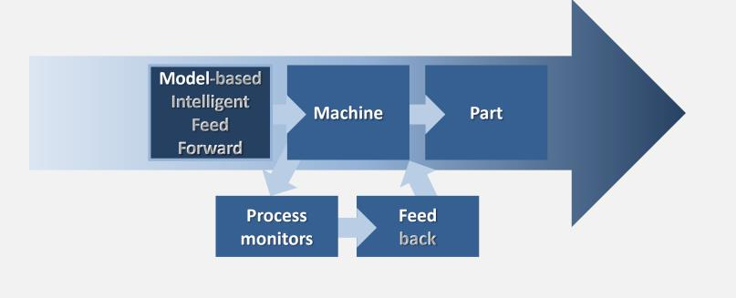
IFF puts a narrow band on parameters and approaches "First time right, every time right" In-situ sensor data can be used to optimize the laser power strategy for challenging geometry features. In particular, it has been shown that pyrometry data is correlated with pore formation. Pyrometry data collected during the print can be used in conjunction with reinforcement learning algorithms to learn an optimal laser power.
