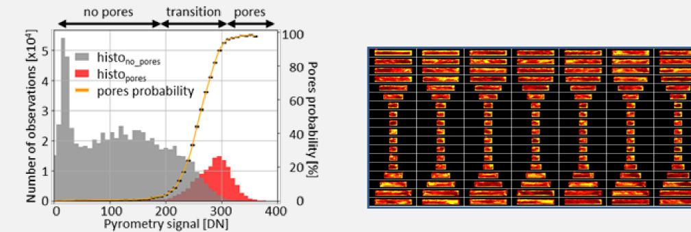
Pyrometry signal is correlated with pore formation Pyrometry signal from dog-bone geometries
