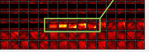
This montage shows the pyrometry signal on different slices of an overhang cube. The pyrometer signal is particularly high at the overhang, where defects are likely to occur.
