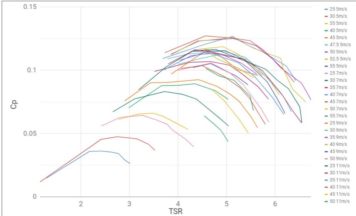
Figure 24.  $C_p$  vs TSR for 2018 test turbine configuration.
