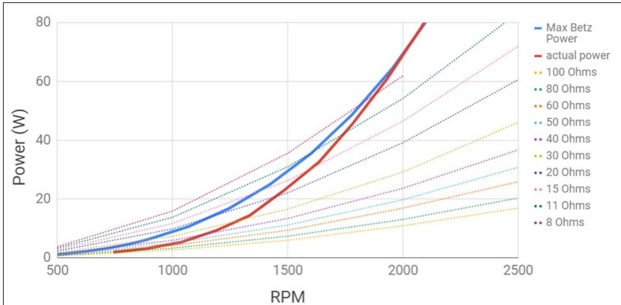
Figure 22: Dynamometer and wind tunnel data for power vs RPM
