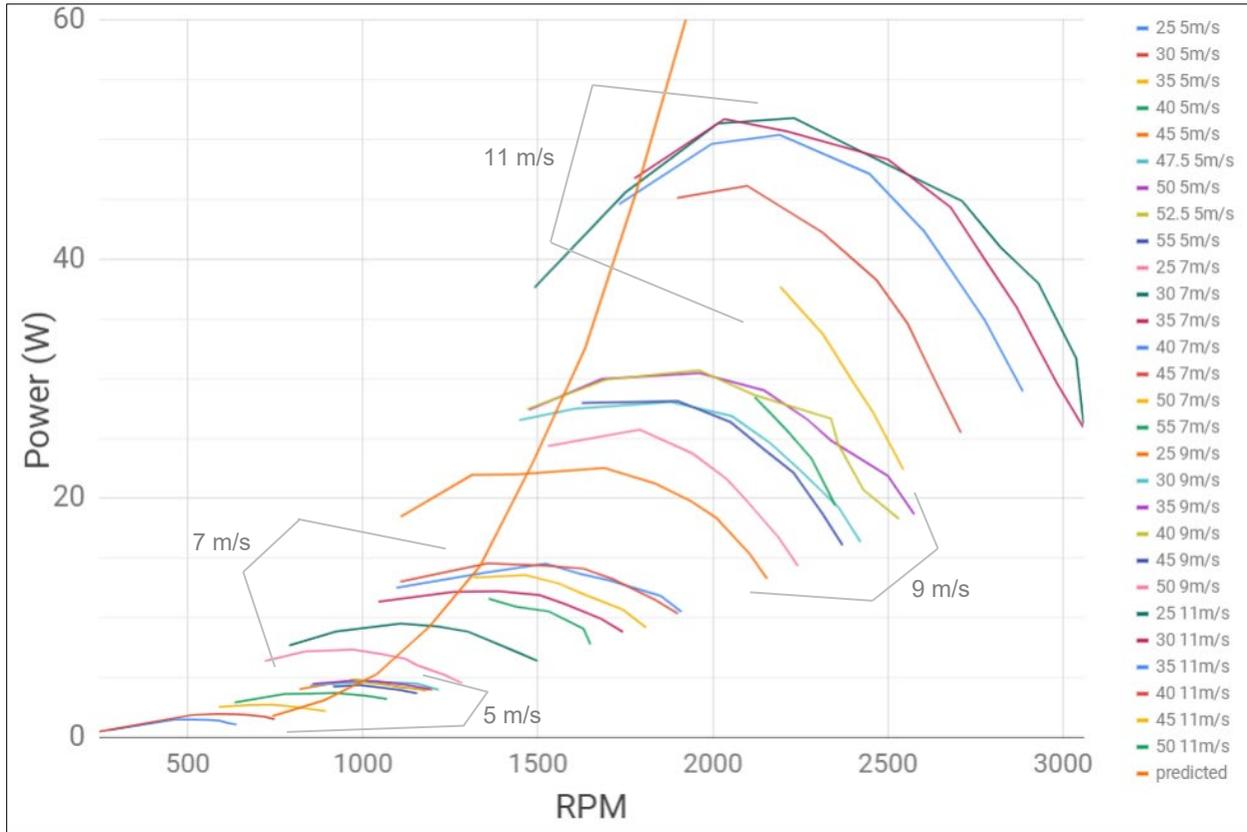
Figure 23: Power produced vs RPM for wind tunnel testing
