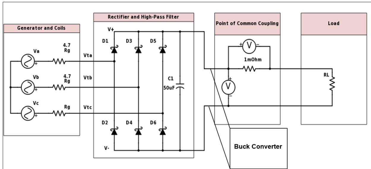
Figure 16: Control circuit and load diagram
