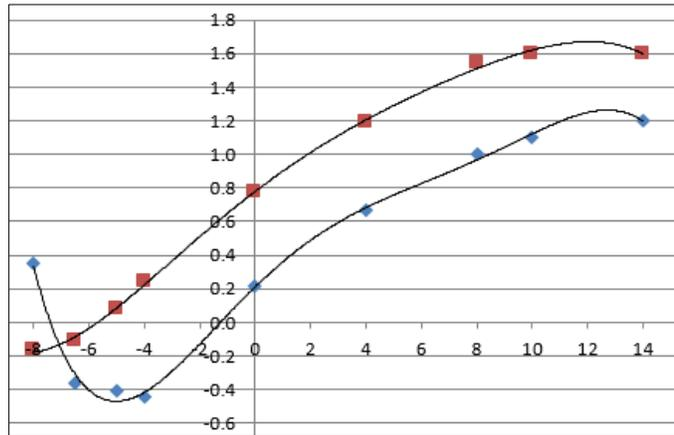
Figure 2: Airfoil  $C_l$  vs Angle-of-Attack for  $Re = 50k$  (Blue),  $Re = 100k$  (Red)
