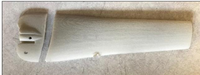
Figure 9: Blade fracture from benchtop strength test
