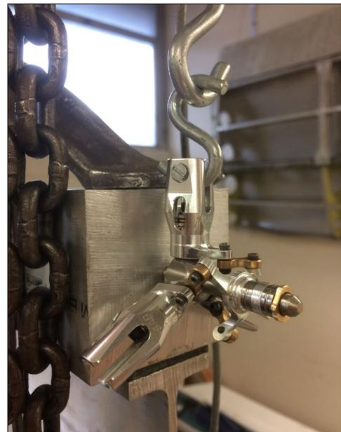
*Figure 12: Blade hub strength test setup*
