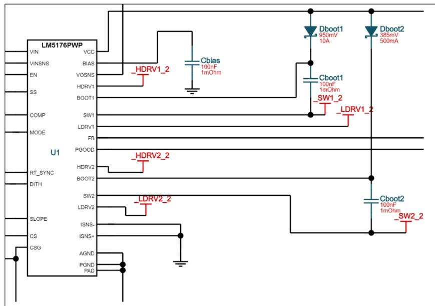
Figure 17: System-level buck converter diagram
