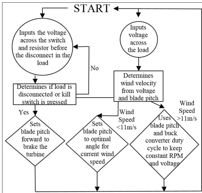
Figure 18: Normal operation control flow chart
