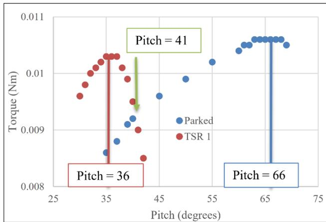
Figure 6: Torque produced vs pitch angle for parked and TSR 1 conditions
