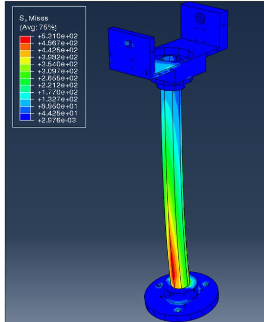
Figure 14: Turbine structure FEA results
