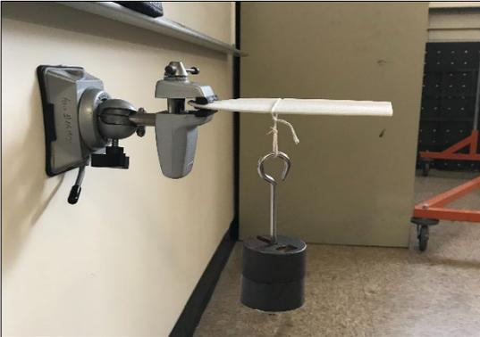
Figure 8: Benchtop blade strength setup
