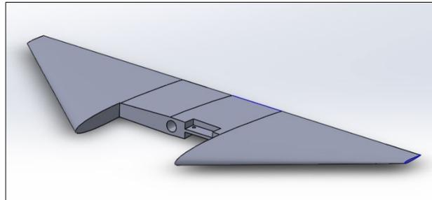
Figure 10: Tailfin with airfoil incorporated
