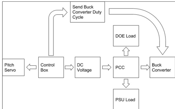
Figure 15: Electrical system control overview diagram
