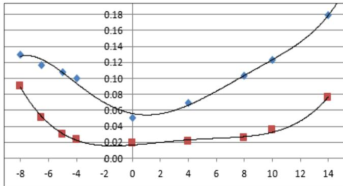
Figure 3: Airfoil  $C_d$  vs Angle-of-Attack for  $Re = 50k$  (Blue),  $Re = 100k$  (Red)
