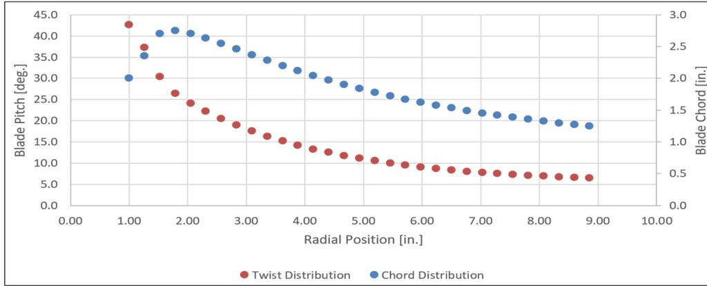
Figure 5: Blade Chord and Twist
