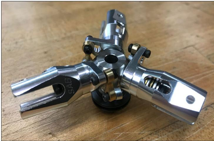
*Figure 11: Blade hub pitching mechanism*
