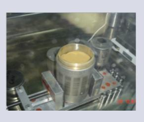
**3.** Pipe cutter opens outer and inner can
