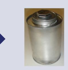
4. Pu oxide is placed in new can along with dry adulterant to dilute Pu to less than 10 weight percent
