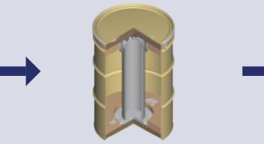
6. Can is removed from glovebox, assayed, and packaged into approved NRC licensed drum
