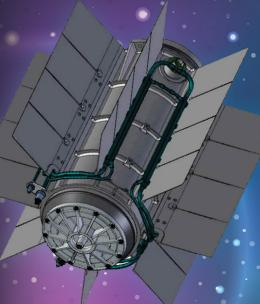
Radioisotope power systems are capable of producing heat and electricity under the harsh conditions encountered in deep space for decades without any maintenance.
