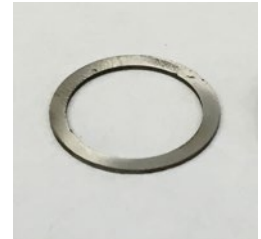
A ring sliced from the consolidated flakes
