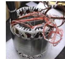
Stator with Winding
