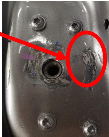
Small Crack on Inner Panel in hinge area
