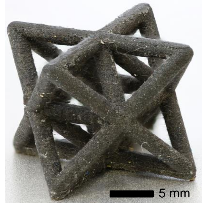
CF octet-truss with \bar{\rho} = 20\%
