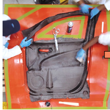
2. Carbon fiber hand layup for vacuum infusion.
