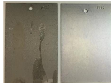
Humidity Test of bare (left) and process D pretreated (right) E-Form Plus sheet shows pretreatment successfully prevented oxidation and corrosion.
