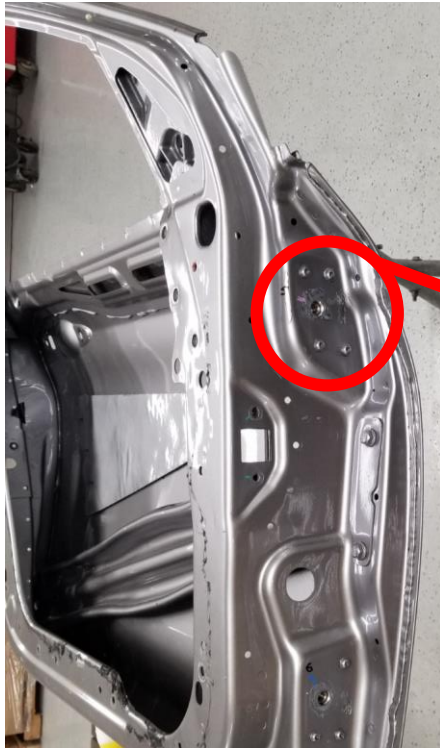
Small Crack on Inner Panel in hinge area
