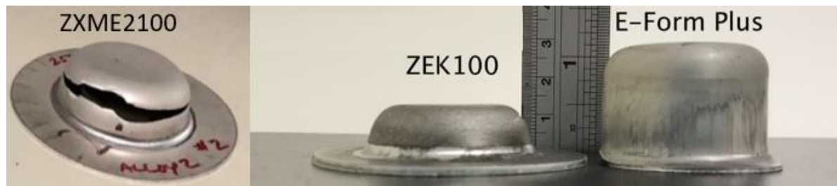
Erichsen cup testing of ZXME2100 (left), ZEK100 (center) and E-Form Plus (right) performed at 250°C shows only E-Form plus was capable for forming the full cup without fracture.
