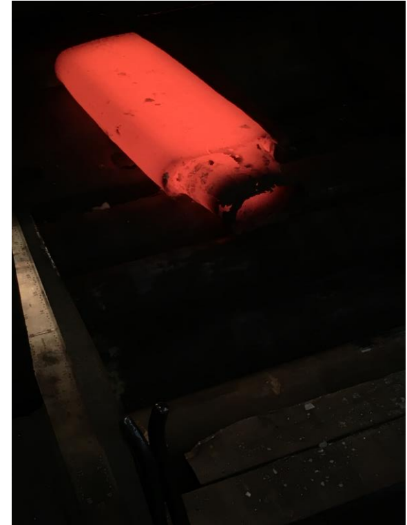
Image of 50 lb heat of ORNL chromia-forming alloy being successfully hot rolled at Special Metals
