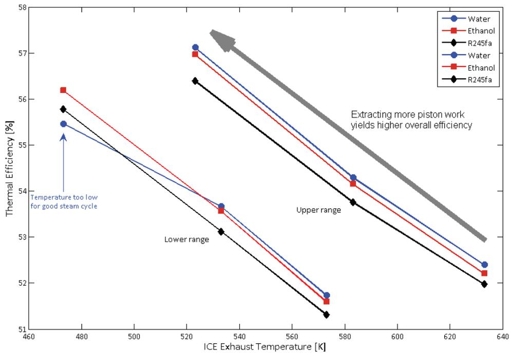
**C:** Stirling-cycle engines have been manufactured that operate in the power range (50–60 kW) suitable for waste-heat recovery (WHR). The lower exhaust temperatures from the RICE limit the efficiency of the Stirling engine, and the overall system efficiency improves with more piston work being extracted. This relationship is shown in Figure 6.D.9, where the higher-efficiency RICE leads to lower-temperature exhaust but overall higher combined system efficiency.
