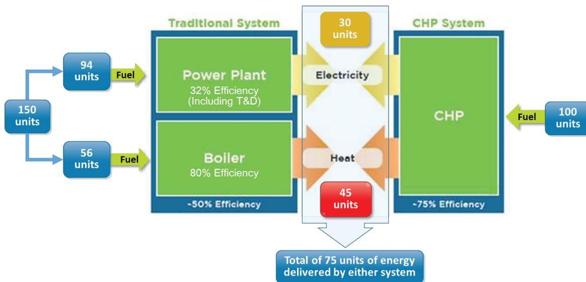
CHP systems can be used in a range of settings and power levels, ranging from multifamily residential and commercial/light industrial systems typically producing as little as 50 kW of power to large industrial systems that produce more than 20 MW of power. Applications include the following:<sup>3</sup>
