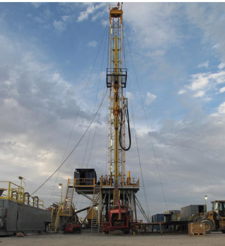
Drilling a 9,000-foot geothermal test hole in Fallon, Nevada.
