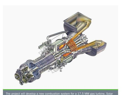
Titan 130, with the goal of enabling the turbine to sustain combustion and avoid lean
