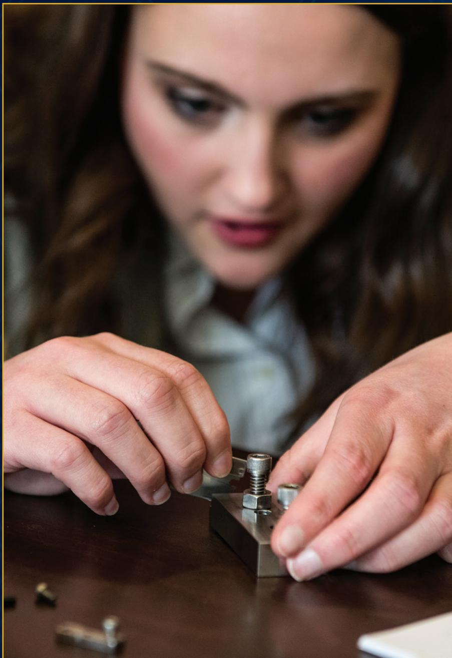
Washington State University student Jacqueline Reeve assembles an apparatus that bends the metal filament to hold samples for thermal ionization mass spectrometer analysis. NNSA's Office of International Nuclear Safeguards Human Capital Development program brings together PNNL safeguards researchers and WSU students enrolled in WSU's Industrial Design Clinic. Photo credit: Maren Disney | Pacific Northwest National Laboratory
