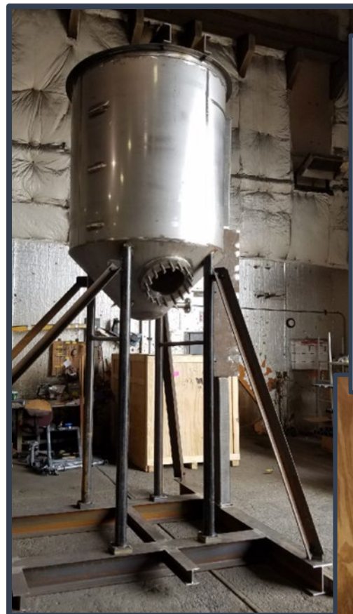
Wet De-con collection and conditioning mockup
