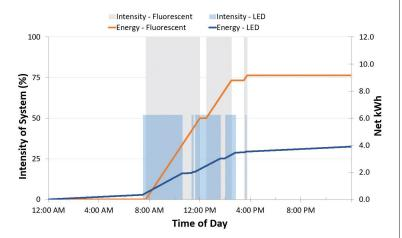
**Figure 3:** Intensity control settings and resulting energy use for a typical day in one of the classrooms in the pilot study. The resulting energy savings during this day for the LED system relative to the existing fluorescent system was 57%.
