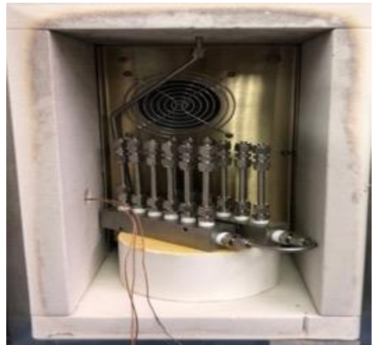
Samples placed in psychrometric chamber
