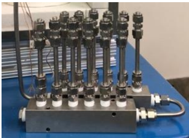
Tube samples placement for thermal and mechanical fatigue tests
