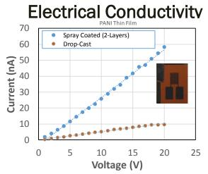
• Linear I-V response measured on PANI thin films deposited on interdigitated electrodes
