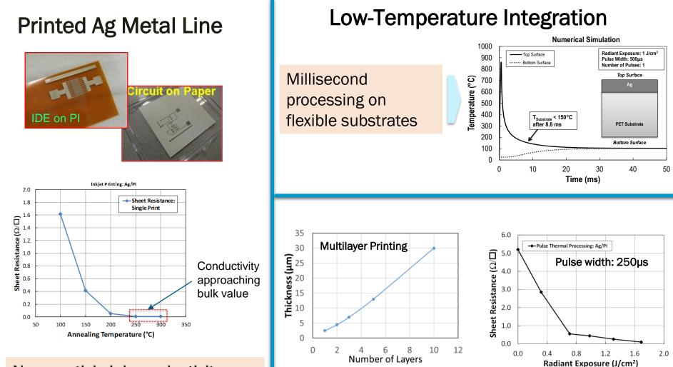
Nanoparticle ink conductivity approaches the bulk value
