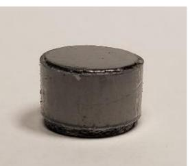
Compressed graphite-salt "puck" before sealing with water vapor impermeable film.
