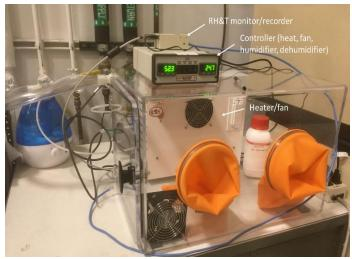
Humidity controlled glovebox for sample transfers
