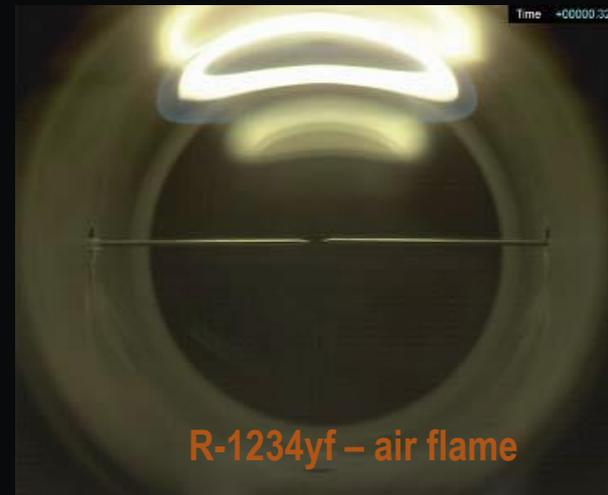
**Flame stretch, radiation heat losses, and buoyancy affect flame behavior. A proper ranking of flammability and an understanding of the full-scale behavior must account for these effects.**
