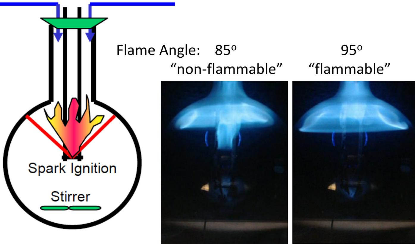
This flammability test depends upon burning velocity (buoyant flow  $\uparrow$ , flame speed  $\leftrightarrow$ )
