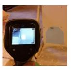
Use IR camera to determine fill rate
