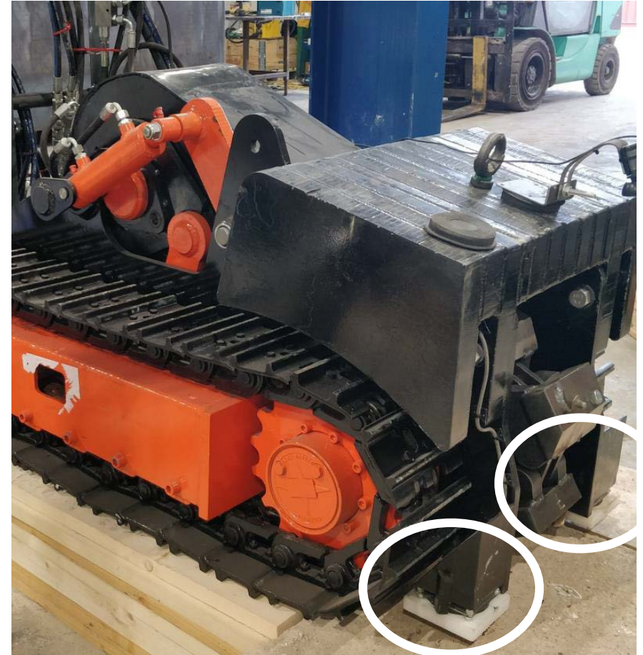
Figure shows Rotocutter at the start of testing, showing both metal detectors with protective nylon cuffs.
