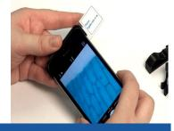
PNNL's mobile Smartphone Microscope allows anyone with a smartphone to explore tiny objects for as little as 5¢. It slips over the smartphone and can be 3D printed.
