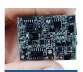
LLNL's MIR is a compact, low-cost, low-power radar used for sensing nearby objects and measuring distances between objects in proximity.
