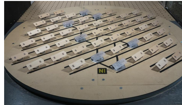
Heliostat Field Wind Tunnel Testing
