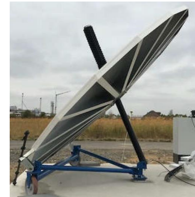
DLR's lay-down heliostat
