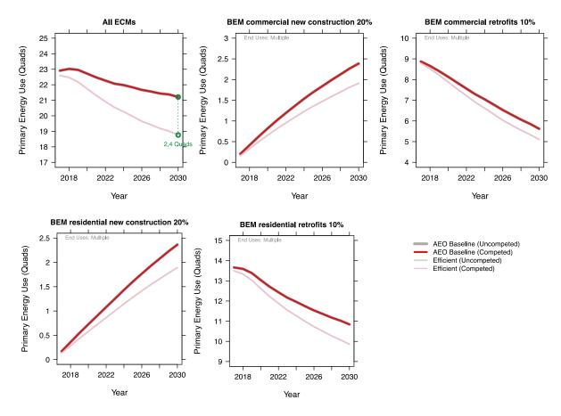
Figure II-5 Scout estimates of potential energy savings due to integrated design and BEM
