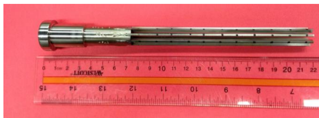
Samples exposed in freeboard of NREL pyrolysis system
