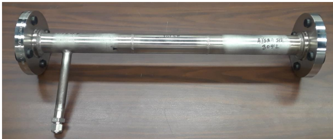
Spool piece exposed in NREL pyrolysis system
