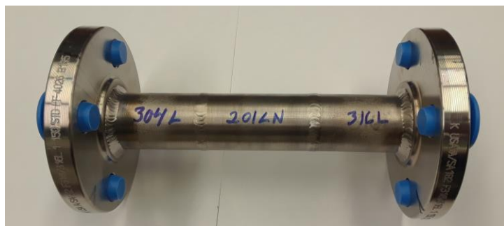
Spool piece exposed in Canmet pyrolysis system
