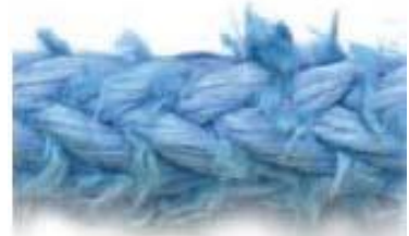
fig. 3 Severely abraded rope
