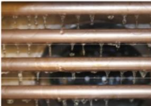
Droplet-Jet mode for falling film evaporator
