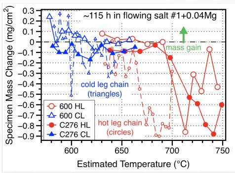
2<sup>nd</sup> loop had 600 and C276 specimens and failed after 115h
