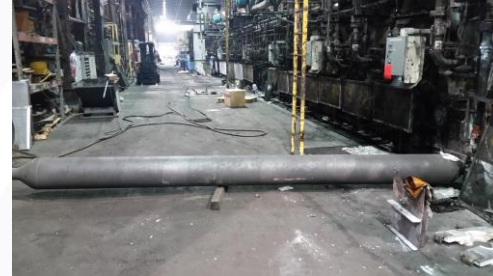
Furnace roll fabricated using centrifugal casting of ORNL alloy has been successfully operating in heat-treat furnace at 900° C for more than two years (ARPA- E OPEN 2015)
