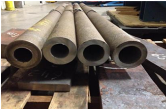
ORNL Alumina Forming Austenitic tubes fabricated using centrifugal casting in air (ARPA- E OPEN 2015)
