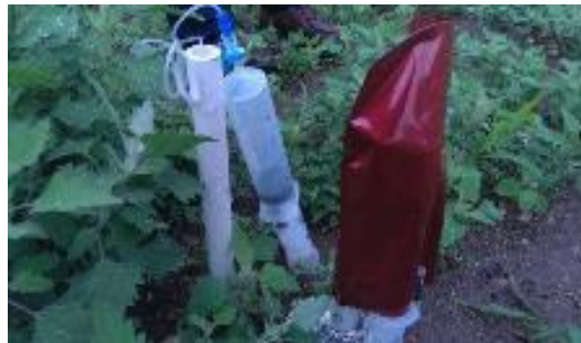
Soil-water sample collectors
