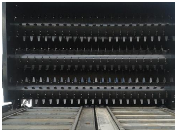
Uneven Flow caused by high speed combined bale processing and size reduction
