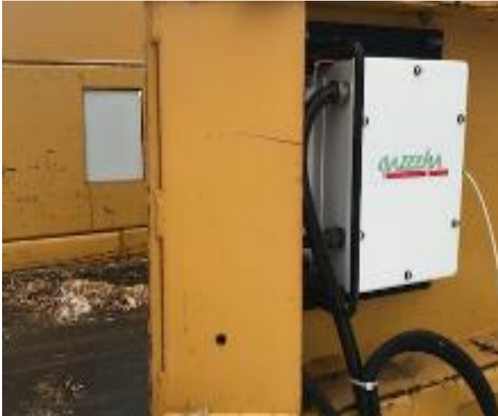
Gazeeka Bale Moisture Sensor on Conveyor feeding the 1st-Stage Grinder
