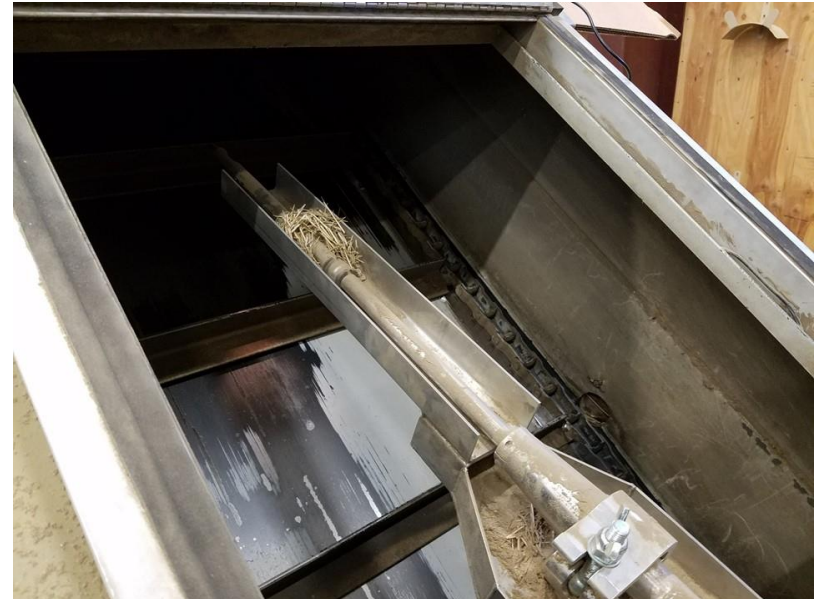
In-line NIR Probe on Drag Chain Conveyor feeding the 2 nd -Stage Grinder.
