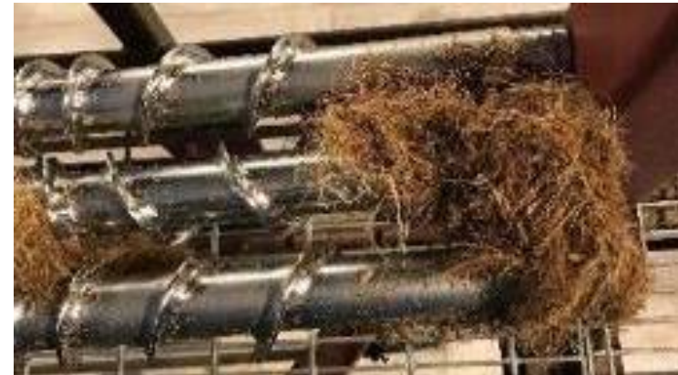
Bridging of Biomass into plug feeder
