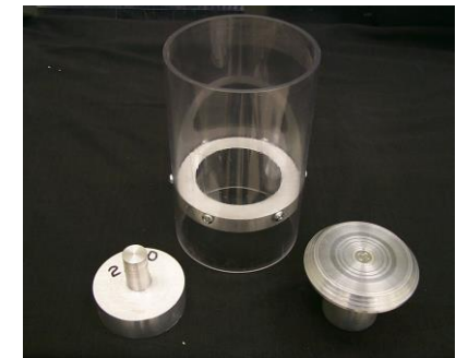
Johanson "extrusion" test
