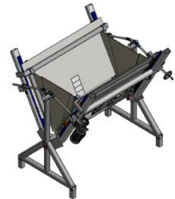
Wedge-shaped hopper with adjustable walls
