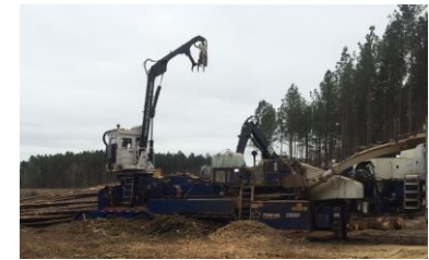
Whole tree disc knife chipper with chain flail
