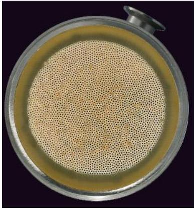
Membrane would quickly become clogged with solids in hydrolysate.
