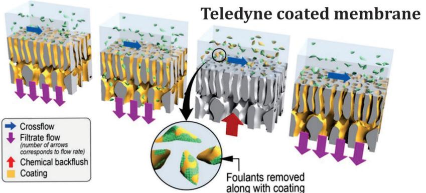
A protective coating (yellow) on the polymer membrane provides chemical and fouling resistance. Removing the foulants and/or coating during chemical backflush and subsequent in-place regeneration increases longevity.
