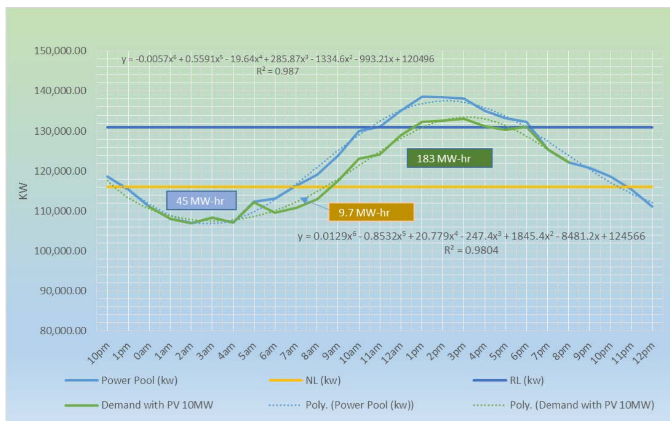
July 2024 Hourly Peak Electric Demand and the potential Peak Demand reduction from a 10MW PV System-Average Day
