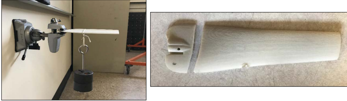
Figure 16: Blade Strength Testing to Failure
