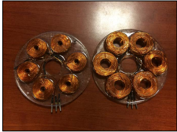
Figure 20: Two Generations of Stators
