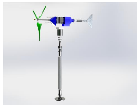
Figure 2-1 Test turbine top assembly exploded view.
