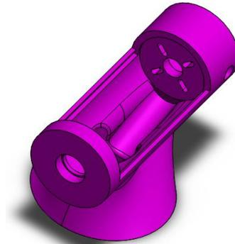
Figure 14. Extra wire space in the bottom of the nacelle
