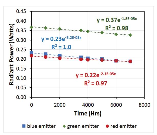
Radiant power determined from the skewed Gaussian curve fits of each spectral emission component of Brite 2 neutral white panels in 450L.
