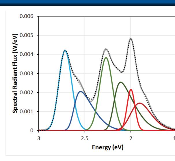
Spectral emission deconvolution of the Brite 2 neutral white panels with two skewed Gaussian used to model each blue, green, and red emitter.
