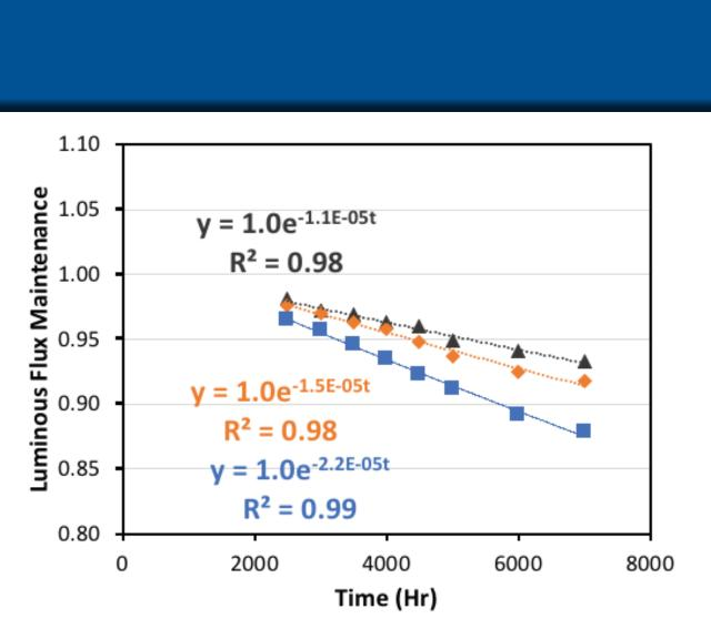
Average luminous flux maintenance for Brite 2 neutral white panels after 7000 hours OL and exponential fits of the latter part of the data.
