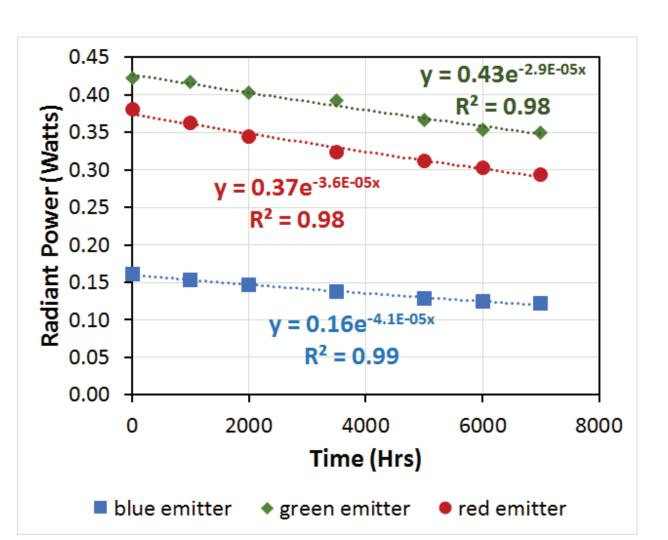
Radiant power determined from the skewed Gaussian curve fits of each spectral emission component of Brite 2 warm white panels in 450L.
