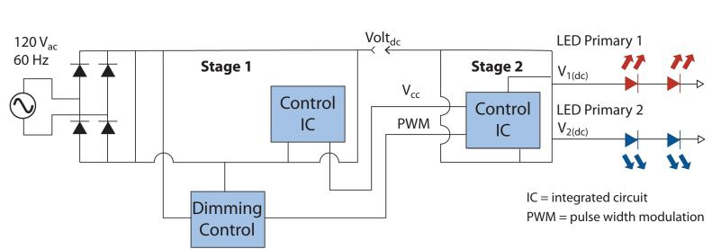
Schematic representation of a two-stage dual-channel driver for operating a TWL system with two LED primaries.
