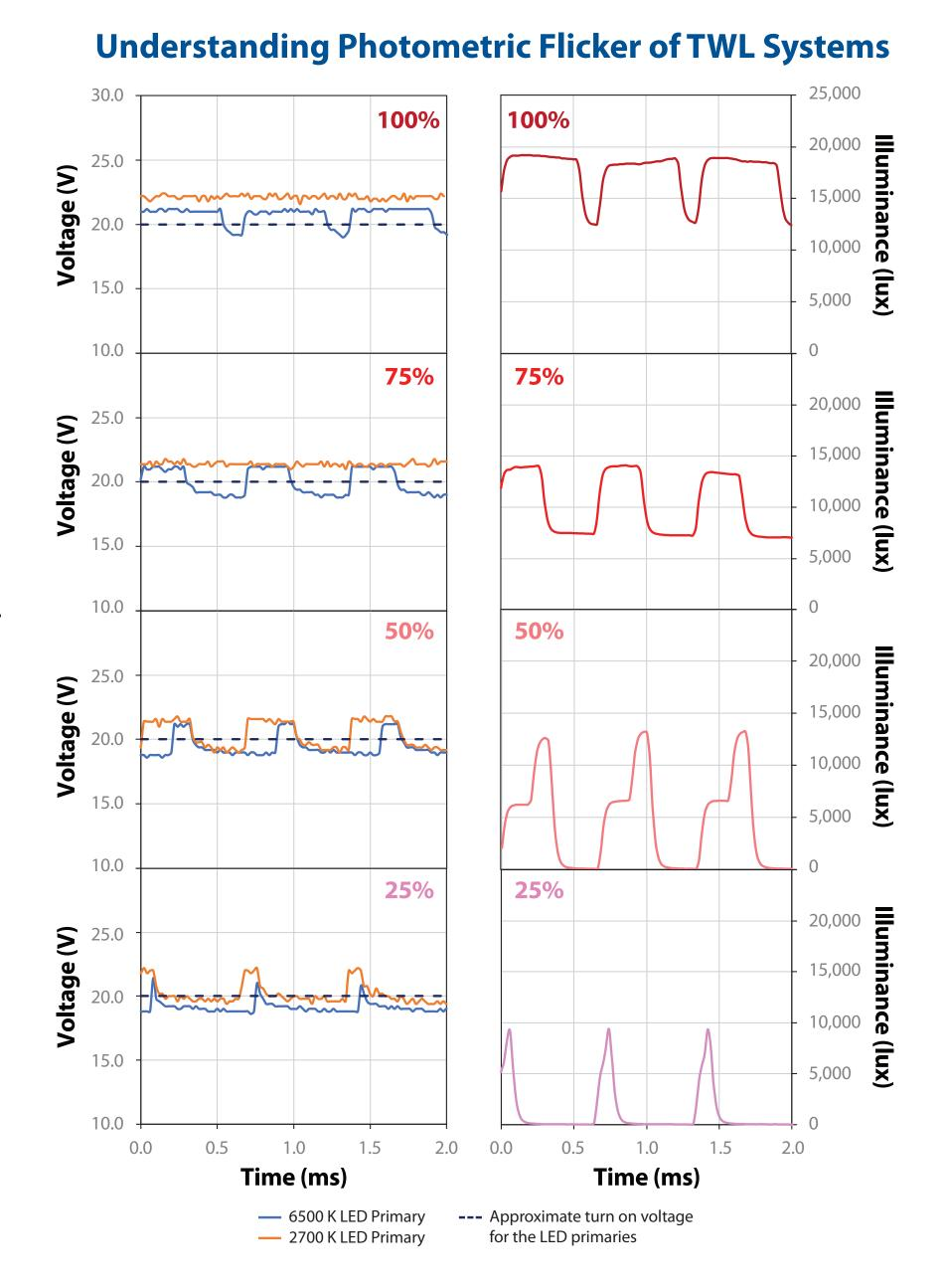
The LED voltage waveforms (left) and corresponding photometric flicker waveforms (right) are shown at various dimming levels (red hue percent labels) for a two-stage dualchannel driver for TWL systems with two LED primaries. The CCT is set to 3,500 K. At 100% (top graphs, maximum power), the two LED primaries operate at different times, but one of them is always on. At 50% dimming (third plots down), the LED primaries have different pulse widths.
