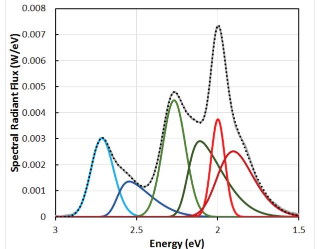
Spectral emission deconvolution of the Brite 2 warm white panels with two skewed Gaussian used to model each blue, green, and red emitter.
