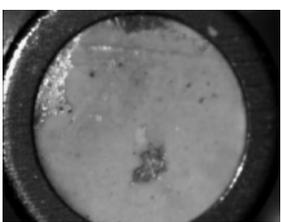
Mg(BH<sub>4</sub>)<sub>2</sub> film on Au for LEIS measurements
