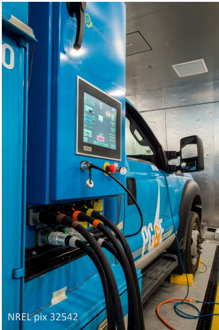
Utility Truck Offering Ability to Power Local Transformers
