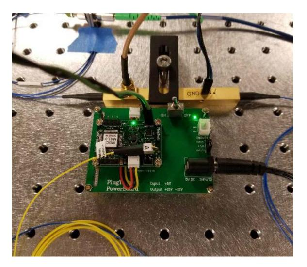
Provides a control voltage to compensate modulator biaspoint drifts.
