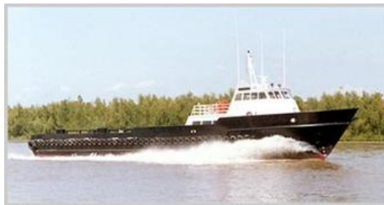
Figure 3-1 Typical crew supply boat
