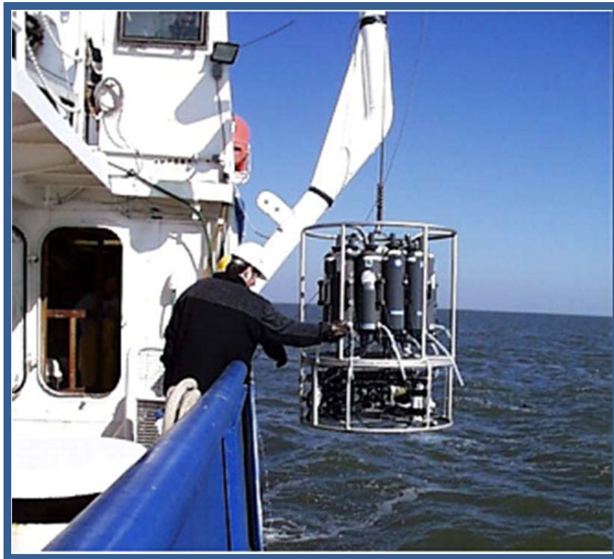
Figure 7 Deploying Rosette Sampler
