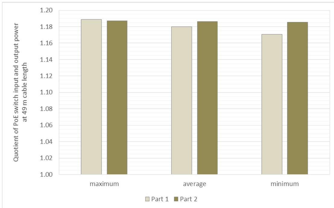
Figure 6. System power (including PoE switch and 49 m cables) relative to combined luminaire input power (4 x 44 W).
