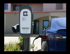
Using the ChargeGuard® is simple: plug the vehicle in, insert the key into the unit, and turn to start charging. The key can be removed and power will be available until the vehicle is disconnected.
