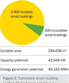
Figure 2. Estimated small building rooftop PV technical potential in Hutchinson, Minnesota. These estimates are available for all cities on SLED. (Source: SLED)
